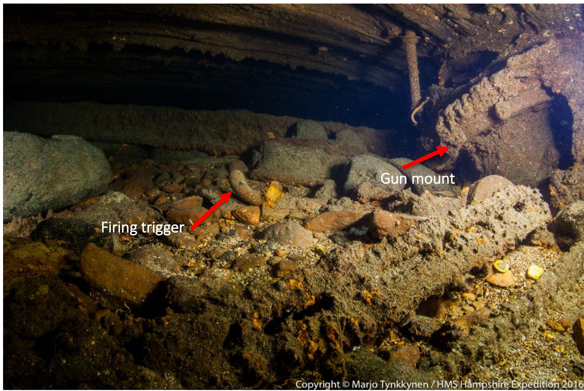
Figure 73: Teak planked deck above. To the right is the gun mount for a Vickers 3-pdr gun
