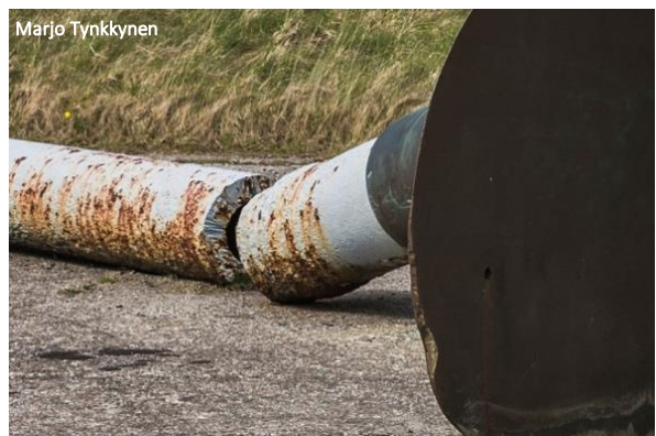
Figure 124: The starboard shaft was cut just aft of the propeller post-salvage
