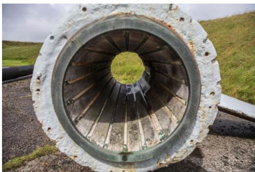
Figure 24: Starboard prop shaft bearing on display at Scapa Flow Visitor Centre & Museum, Lyness
