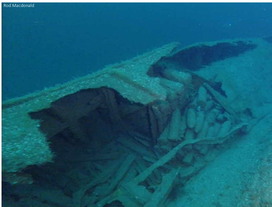
Figure 102: A view from forward, looking aft of the port 6-inch shell room showing separation and collapse of hull bottom (right) from port side of the ship (left)
