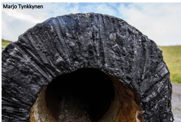
Figure 124: The starboard shaft was cut just aft of the propeller post-salvage
