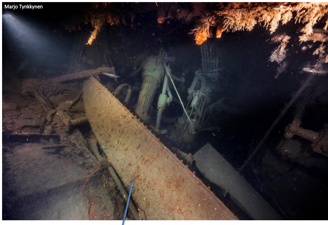
Figure 79: The aft end of the port bilge keel is visible in the fissure lying alongside evaporators
