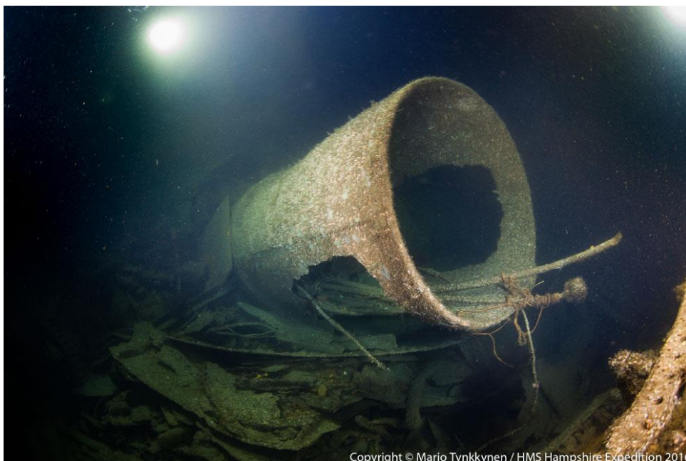
Figure 48: Looking aft on the starboard side at the base of A-turret hoist trunking
