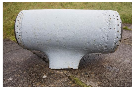
Figure 24: Starboard prop shaft bearing on display at Scapa Flow Visitor Centre & Museum, Lyness
