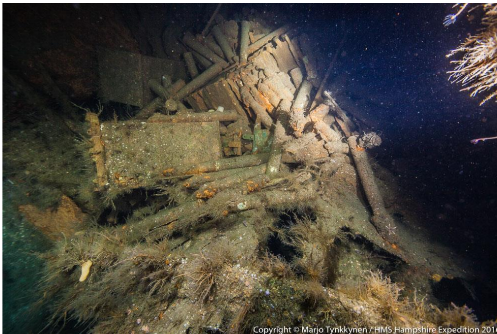
Figure 103: Vickers 3-pdr QF ammunition abaft Y-turret, directly under the port prop shaft
