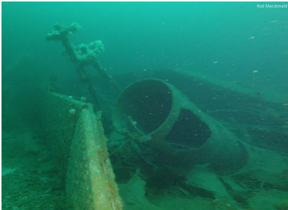
Figure 47: Starboard waterline vertical armour belt plates to left of shot, with A-turret ammunition hoist trunking in foreground and capstan drive shafts and gearing beyond
