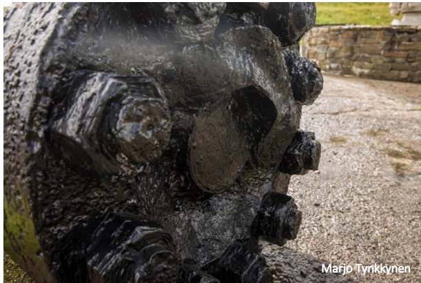
Figure 123: The broken flange joint of the starboard side prop shaft housed at Sapa Flow Visitor Centre
