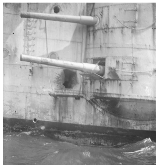
Figure 87: Stern port-side double casemate, as seen here on HMS KENT
