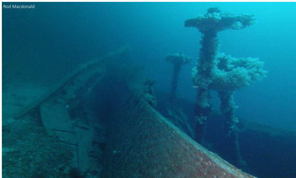
Figure 44: Wide angle starboard view of severed keel
