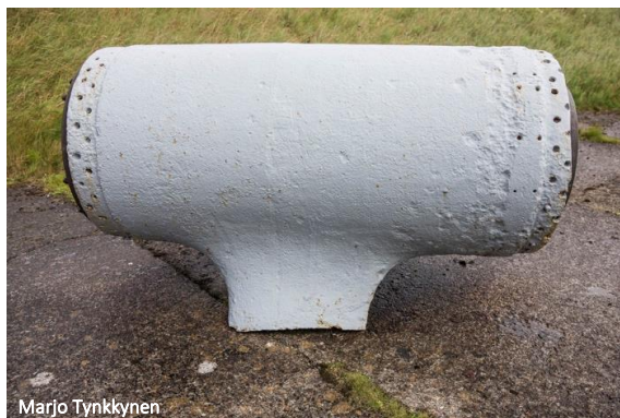
Figure 127: Starboard side A-frame bracket showing the severed short arm
