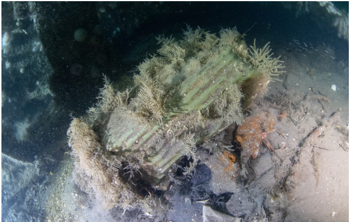
Brass corrugated flash proof container holding bagged cordite charge for forward 5.5"/50-cal BL Mark I deck gun. © Rick Ayrton
