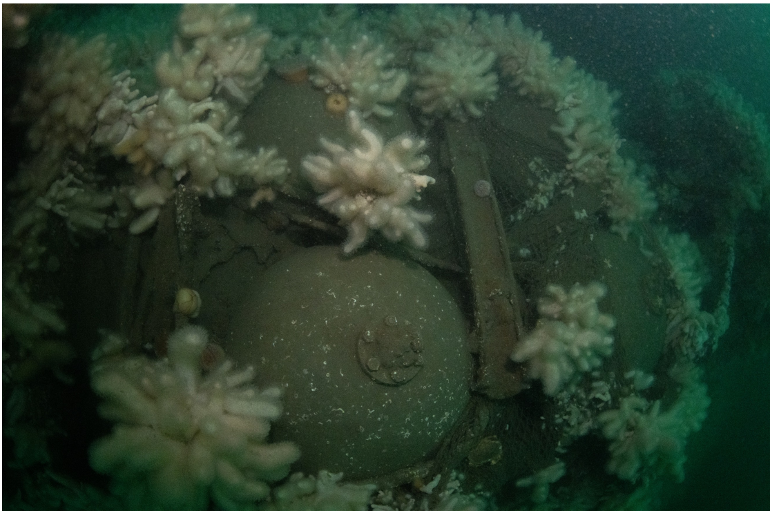
View of all four boiler room ventilator mushroom seals in closed position.
