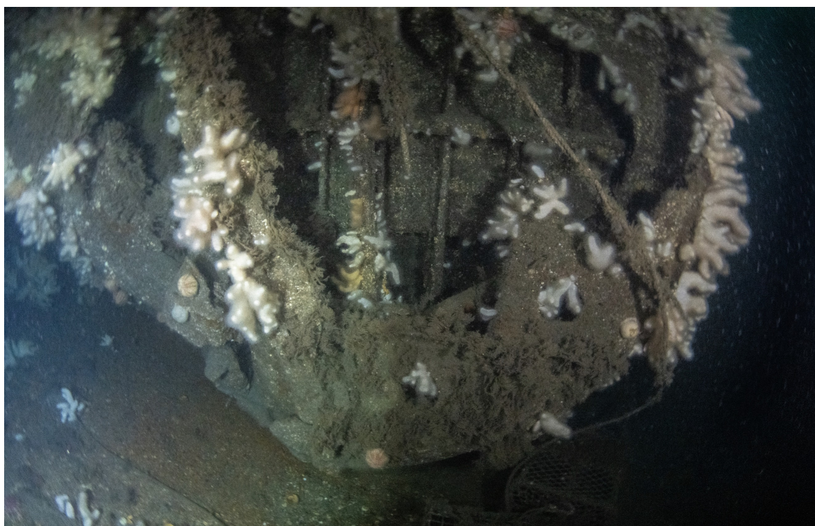
ABOVE & BELOW. Looking aft from free water (where the Officers' Quarters would have been) forward of the break point towards the bulkhead at Frame 160 that formed the aft bulkhead of the Officers' Quarters. The bulkhead is intact. © Rick Ayrton
