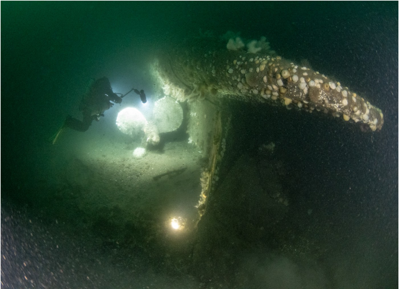
The delicate fantail of K 17 with half buried rudder and port propeller – the diver gives scale.
