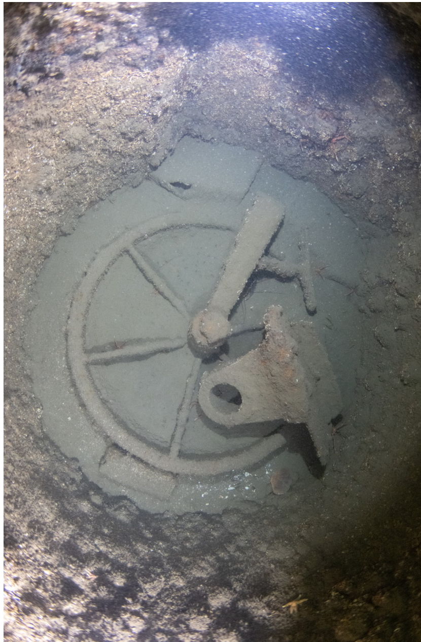
The lower hatch of the No. 2 (after) funnel boiler room uptake is in the closed position.
